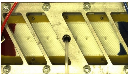
Figure 5.25: Visualization of in-plane impregnation strategies with different materials: parallel impregnation
