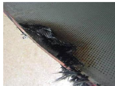
Figure 1.7: A generic thrust reverser panel with lightning strike damage [15]
