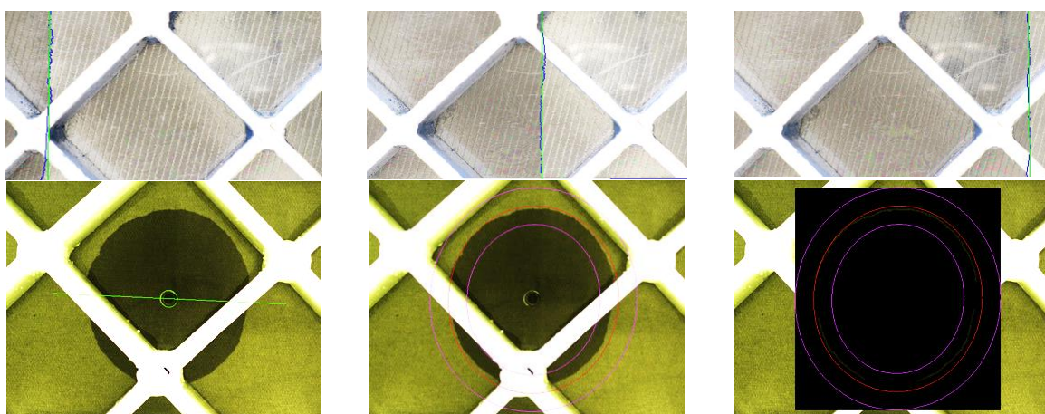
Figure 3.21: Example image of a 1D linear flow (top) and 2D radial-flow (bottom) experiment and evaluation steps of the digital image processing algorithm (left to right)
